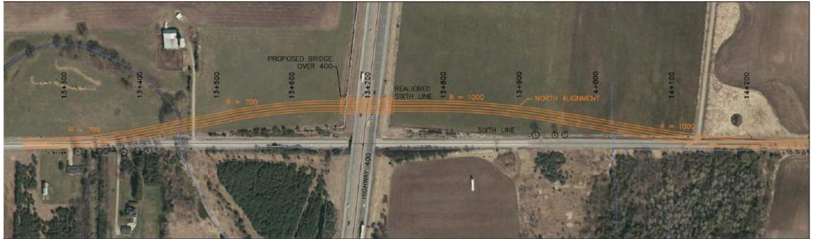
Figure 5.3: Horizontal Alignment Alternative B
