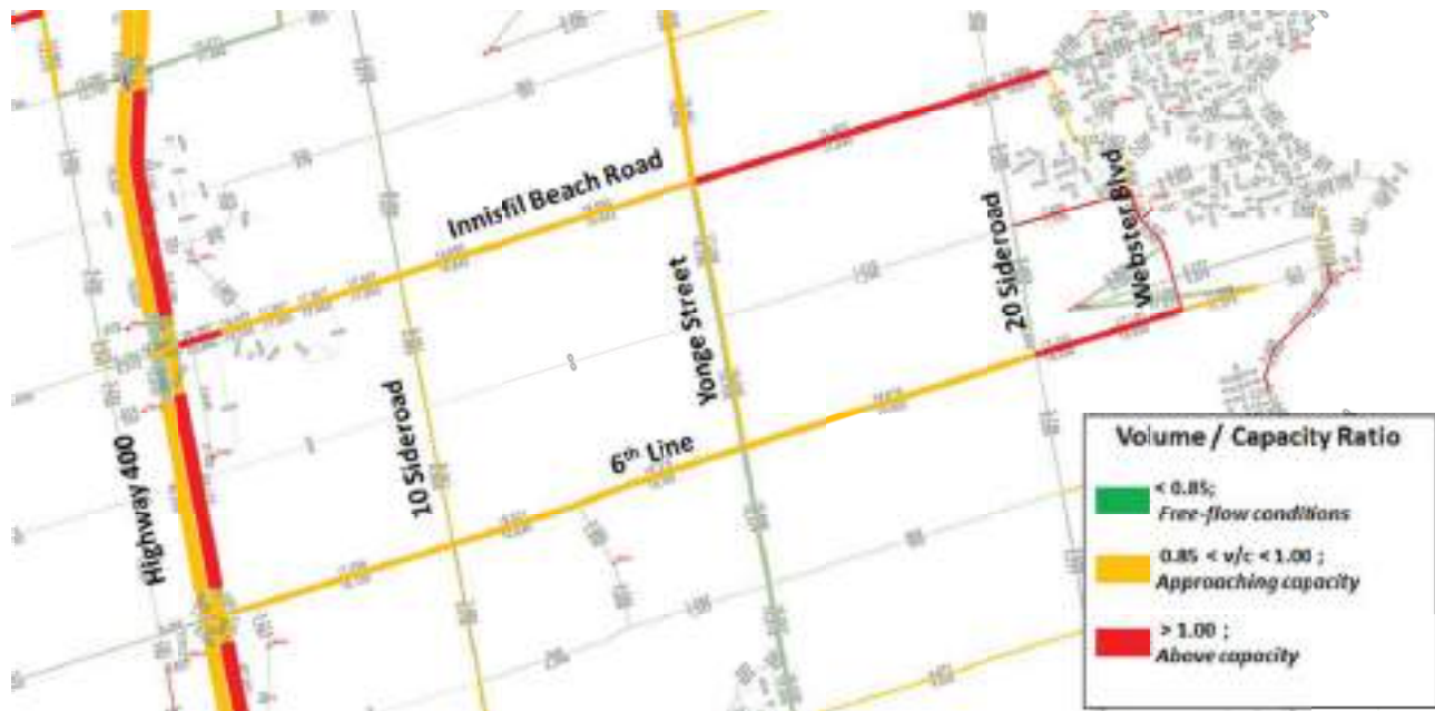
Exhibit 13: Scenario 5 – Widening with Capacity and Speed Improvements Auto Volume and Volume / Capacity Results
