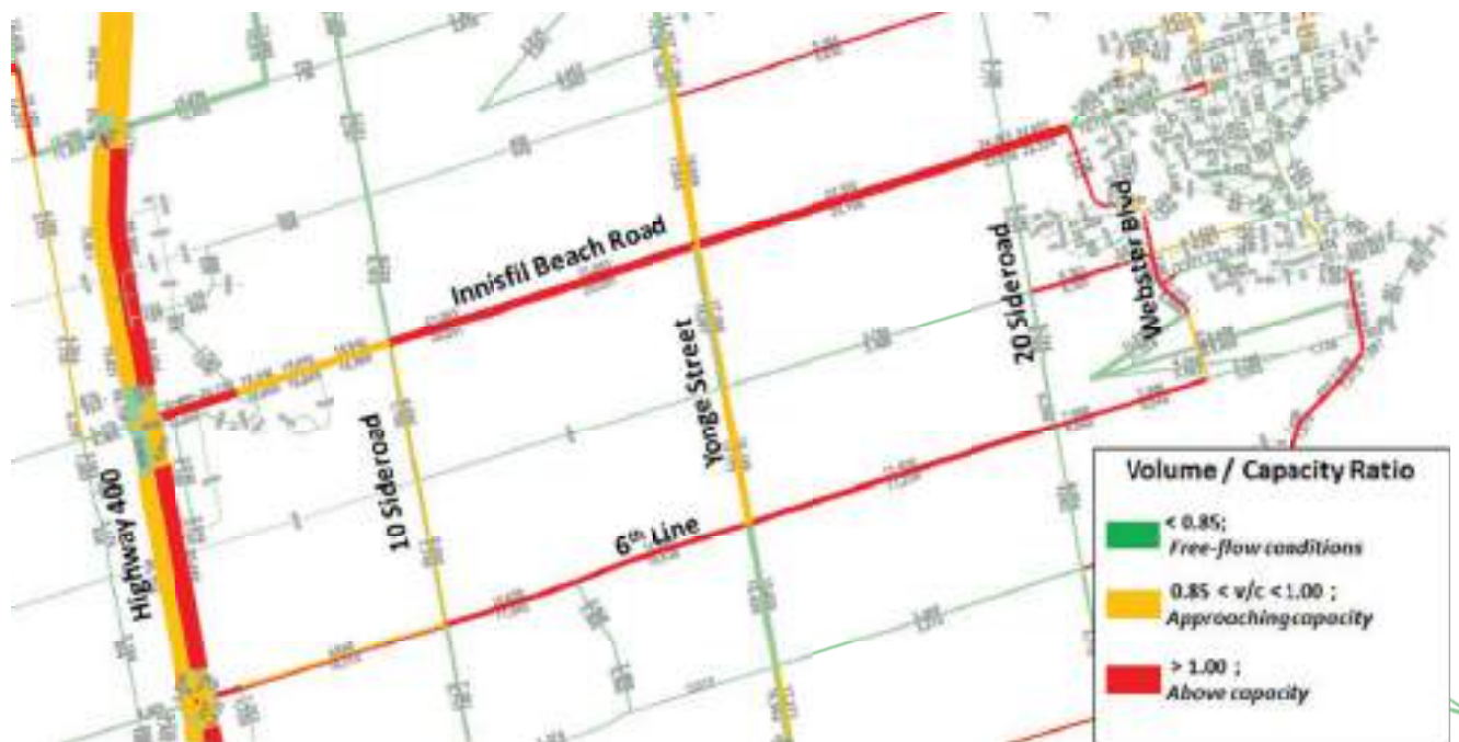
Exhibit 12: Scenario 4 - Capacity and Speed Improvements with Highway 400 IC Auto Volume and Volume / Capacity Results
